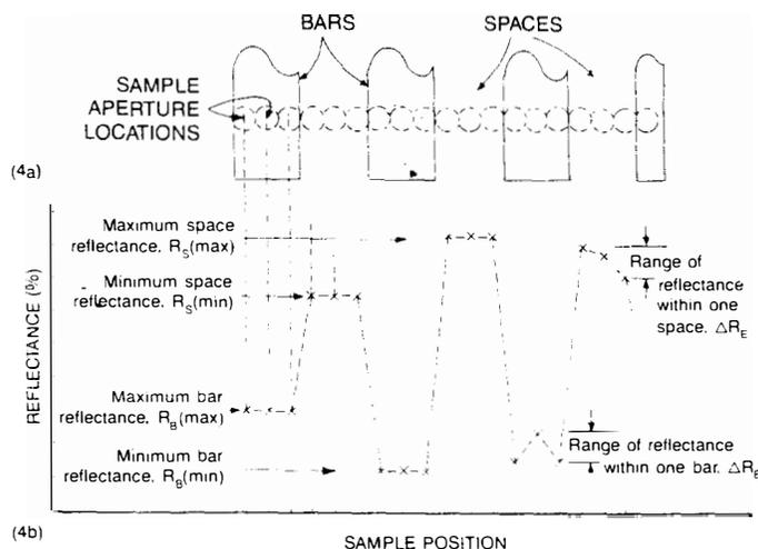
Figure 4. Bar Code Reflectance Measurements
