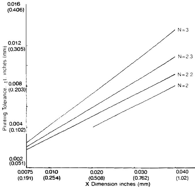
Figure 3 USS-39 Dimensional Tolerances
