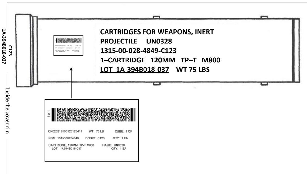
FIGURE 47. Identification marking and the placement of ammo/explosives identification bar code labels for exterior cylindrical containers.
