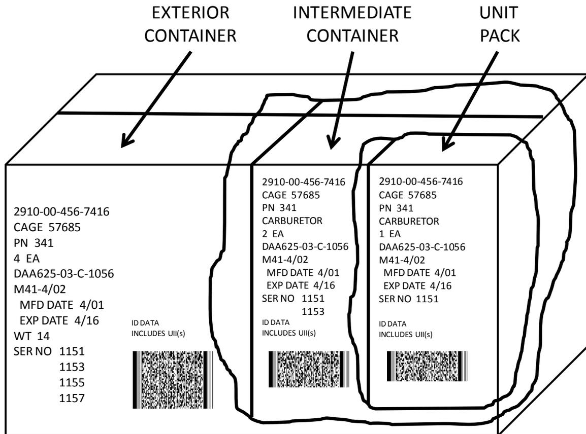
NOTE: For hazardous marking, see 5.13. Linear bar codes are optional when the 2D (PDF417) bar code includes the identification data.
