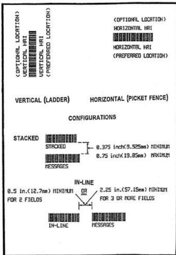
FIGURE 16A. Linear (Code 39) bar code configurations.
