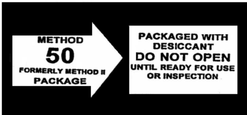
FIGURE 31. Method 50 marking.
